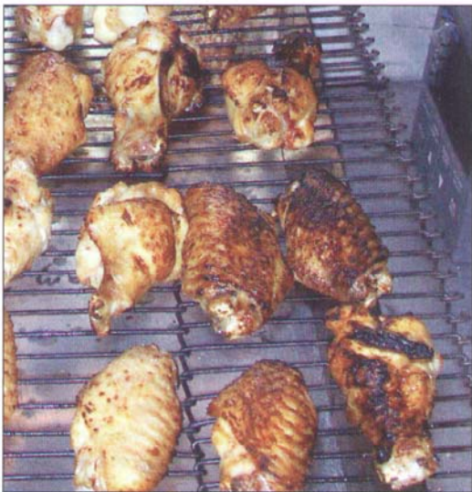
Fig. 6: A conveyor carries the product to be browned under the IR burners at high speed. Pyramid Food Processing Equipment Manufacturing, Tewksbury, Mass.
