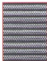
Photo of section of ceramic refractory grid.
